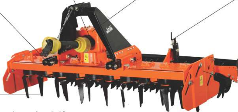
Universal joint power transmission shaft with shear bolt torque limiter
