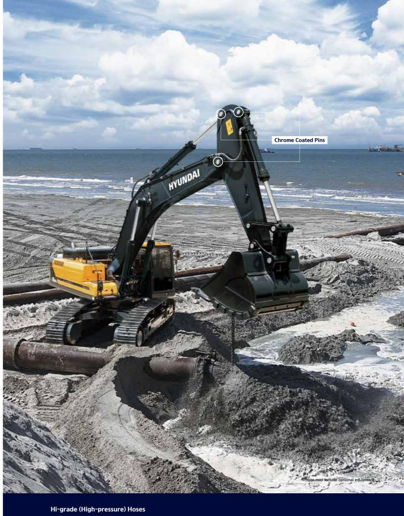
The HX Series uses high-pressure hoses with improved heat and pressure resistance, greatly increasing the durability of the equipment.
