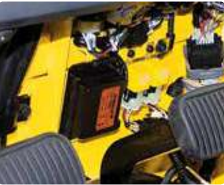
Improvement in Maintenance of Electric Parts Various electric parts are centralized in dash board resulting in effortless troubleshooting.
