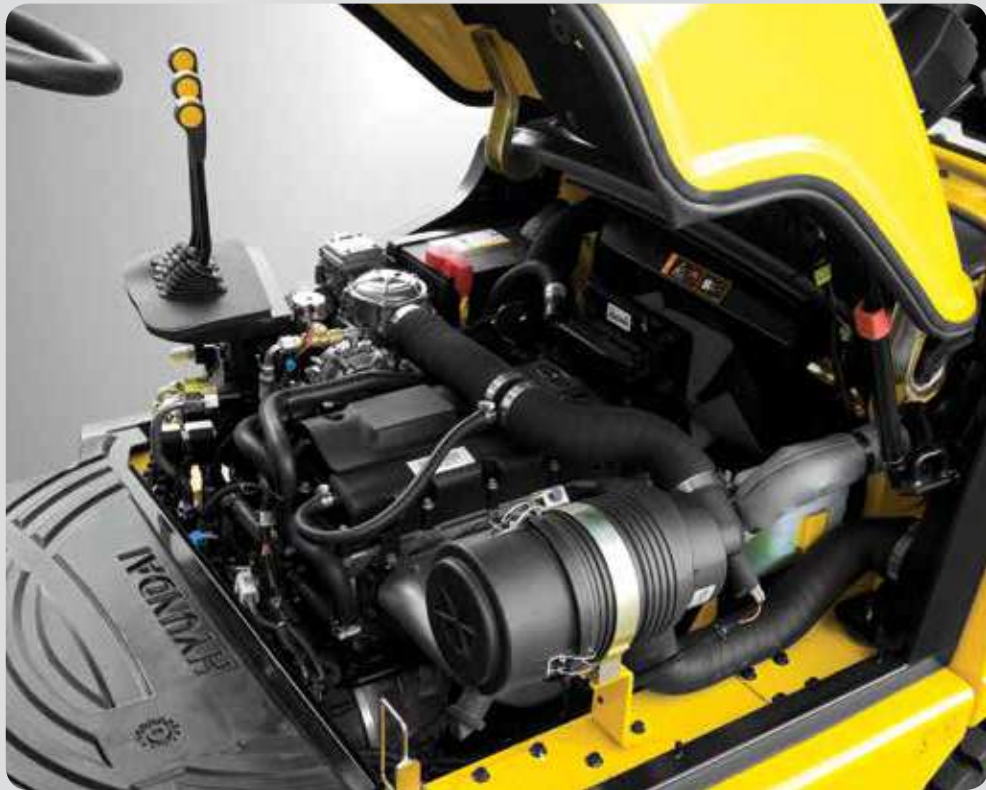
Easy Change Air Cleaner The air filter is readily accessible for cleaning or replacement. (6inch Cyclone Type)
